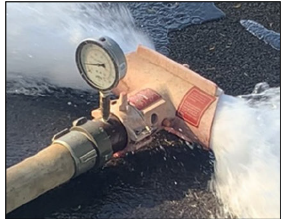
Figure 6-13 Pitot Pressure Reading
